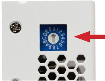
USE A FLATHEAD SCREWDRIVER TO TOGGLE BETWEEN DIFFERENT PRESET EDIDS BY TWISTING THE DIAL TO THE PREFERRED EDID. THE FOLLOWING CHOICES ARE AVAILABLE:
