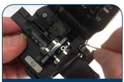
1. Using the Allen wrench included with the cleaver, on the top right side remove the screw that secures the fiber scrap box. Set the scrap box aside. \*Varies by model.
