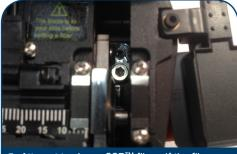
Attempt to cleave SSF<sup>™</sup> fiber. If the fiber does not successfully cleave repeat Blade UP steps A & B to increase blade height until a successful cleave is achieved, reassemble.
