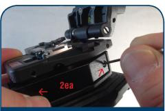
Using the Allen wrench remove the two screws that secure the guide cover.\*Not all models.
