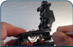
4. Loosen the guide screws with the supplied wrench. Only approx. one turn is required, do not loosen completely.
