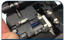
5. Cleave fiber measuring from fan tubing. For SSF<sup>TM</sup> LC = 12mm.  $^{2}$
