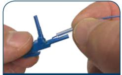
Slide build tube forward and seat in rear of connector, ensure fiber is straight, close hinge. Slide boot forward and tighten until secure.
