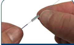
2. Slide included 900µm build tube section onto fan tubing.
