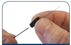
1. Ensure a minimum of 50mm of fiber exits the fan tubing. Unscrew boot from rear of connector and slide onto fan tubing.
