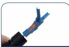
3. Place onto VFL using an LC type adapter. Ensure activator slide tab is in "open" position - slide towards rear of connector. Open hinge on connector.
