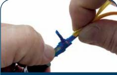
7. Slide activator tab towards connector tip. Remove from VFL. Ensure fiber is straight, hold Kevlar to one side (2.0mm seat tube at rear of connector). Close hinge.
