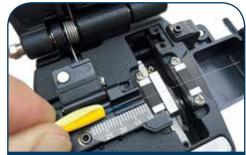
5. Cleave fiber measuring from cable jacket. For SSF<sup>m</sup> LC = 24mm.<sup>2</sup>
