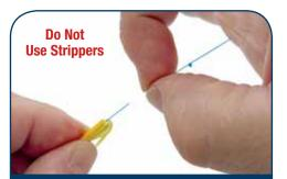
4. Pull Kevlar yarns back to locate SSF™ fiber. Use only finger tips/nails to gently remove "Soft Peel" 250um coating to within 12mm/1/2" of cable jacket. 1
