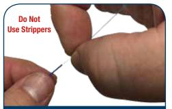
Use only finger tips/nails to gently remove "Soft Peel" 250µm coating completely to fan tubing.<sup>1</sup>
