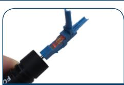
3. Place onto VFL using an LC type adapter. Ensure activator slide tab is in "open" postion - slide towards rear of connector. Open hinge on connector.
