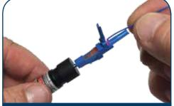
Insert fiber into the rear of connector until a slight "bow" is created and the light emitting from connector window dims and/or extinguishes.
