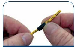
1. Unscrew boot from rear of connector and slide onto cable jacket. For 2.0mm slide included build tube onto cable jacket.
