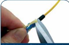
8. Install dust cap. Slide boot forward and thread one full turn to "lock in" Kevlar strands. Cut Kevlar close to boot. Tighten boot until secure.
