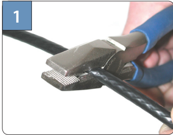
Cut cable squarley.
