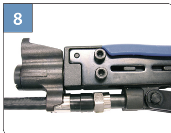
Properly seat connector and compress fully.
