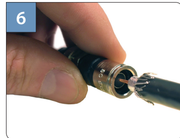
Guide center conductor and dielectric into post. Insert cable into connector until dielectric is flush within post.
