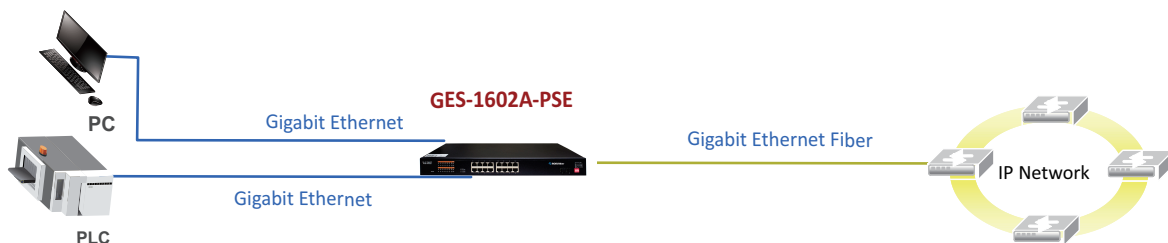
GES-1602A-PSE Gigabit Ethernet Switch Application
