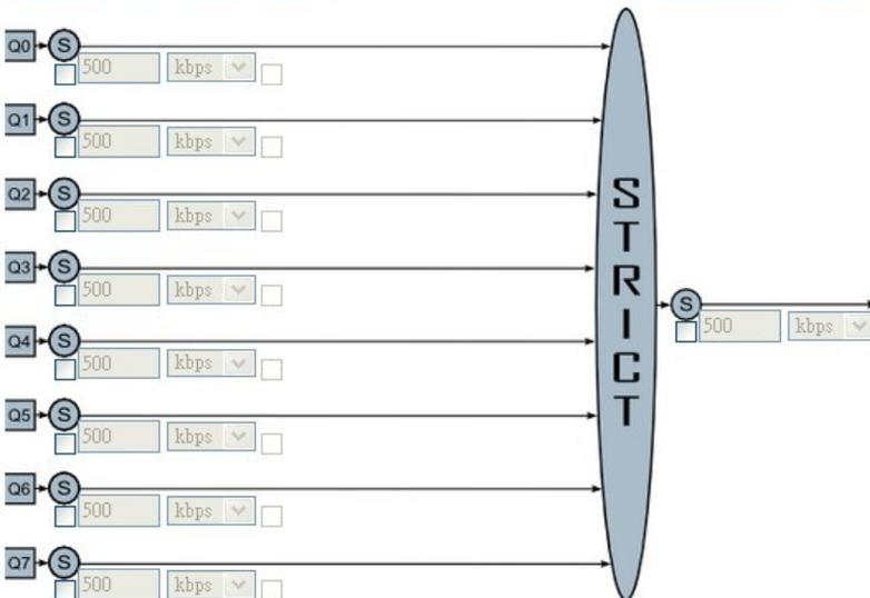
The traffic scheduler could operate in Strict Priority mode or Weighted mode. If in Weighted mode, the weighting of each queue could be configured.
