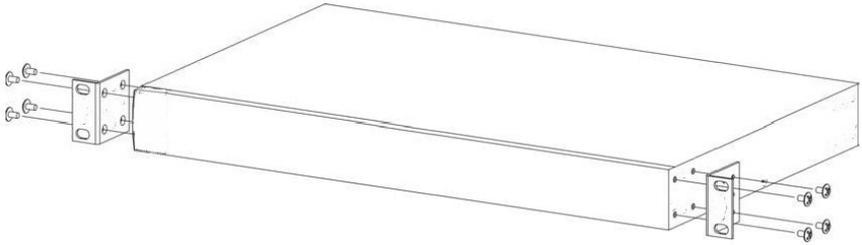
1. Position a Rack-Mount Bracket on one side of the Switch.
