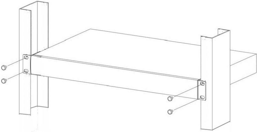
1. Position a bracket that is already attached to the switch on one side of the rack.
