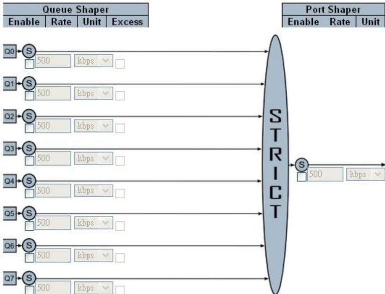
The traffic scheduler could operate in Strict Priority mode or Weighted mode. If in Weighted mode, the weighting of each queue could be configured. The traffic shaper could operate by queue or by port. Enable by checking it and
