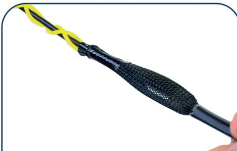
5. When the cable is under tension, the strength members will cinch down onto the cable while keeping the connectors protected.
