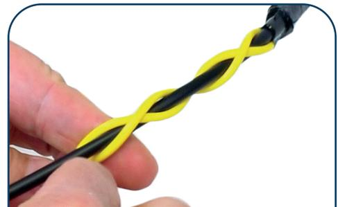
3. Braid the yellow strength members down the cable. Alternate crossing the two legs of the tubing above and below the cable.
