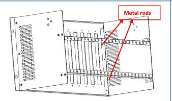
**Step 4.** Install the two metal rods with screws (3\*6mm).
