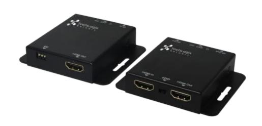
The TL-TP50-HDIR is a cost-effective twisted pair extender set designed for extending HDMI and IR up to 50 meters (164 ft.) over shielded twisted pair cabling (shielded connectors are also required). The system transmits IR from the destination (receiver end) to the source (transmitter end), and requires power on both ends. The transmitter features a built-in loop out, allowing a local display to be connected to the system.
