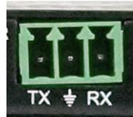
This is how the cable should look. If using the AC-CABLE-3.5-DB9F (Female) or AC-CABLE-3.5-DB9M (Male), the colors will be the same. With any other cable, please follow Tx, G, Rx as shown above. A RS-232 cable preparation diagram is on the next page.
